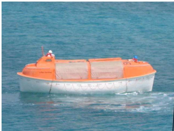
Lifeboat waterborne, released from blocks and manoeuvred
